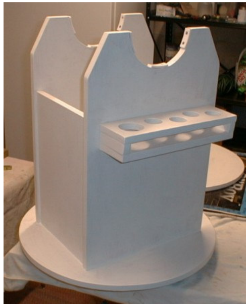
Assembled base—These pictures are of the base after it was primed. The eyepiece holder and bottom circle are visible in the second picture.
