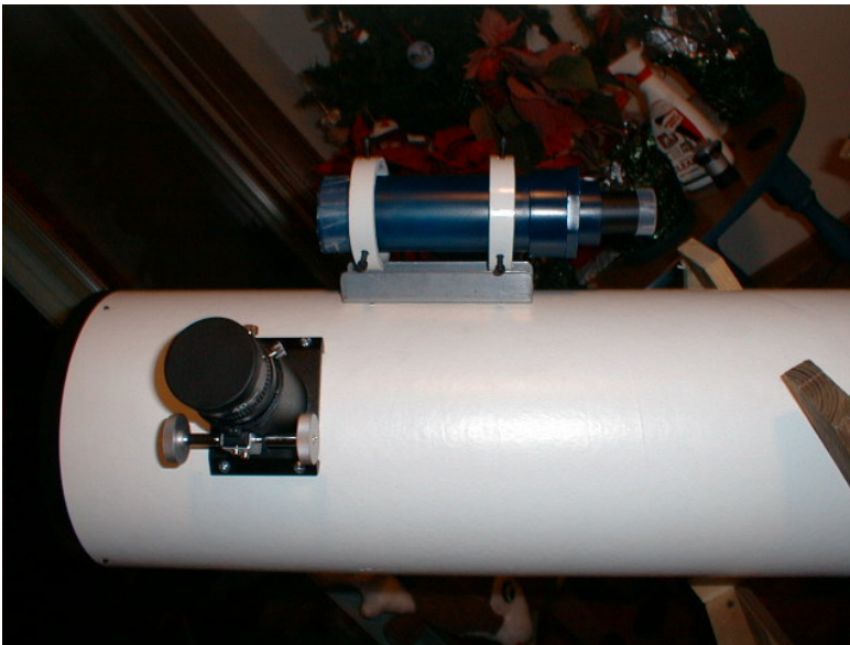
Completed Finder Scope and Holder → Two \frac{3}{4} inch cylinders of PVC pipe are attached to a metal bracket which is attached to the tube. Three screws are placed into three holes that were drilled to hold the Finder Scope center.
