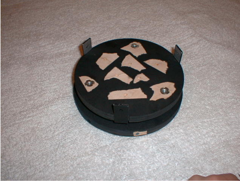
Incomplete mirror cell – The mirror will sit on the top circle and be glued to the wood and aluminum brackets that are screwed to the circle. The top circle is attached to the bottom, larger circle by three “bolt / spring” assemblies.
