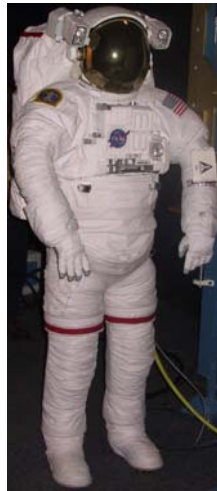
Figure 1-4 Extravehicular Mobility Unit (EMU) Suit Visual (Ref. [1])
