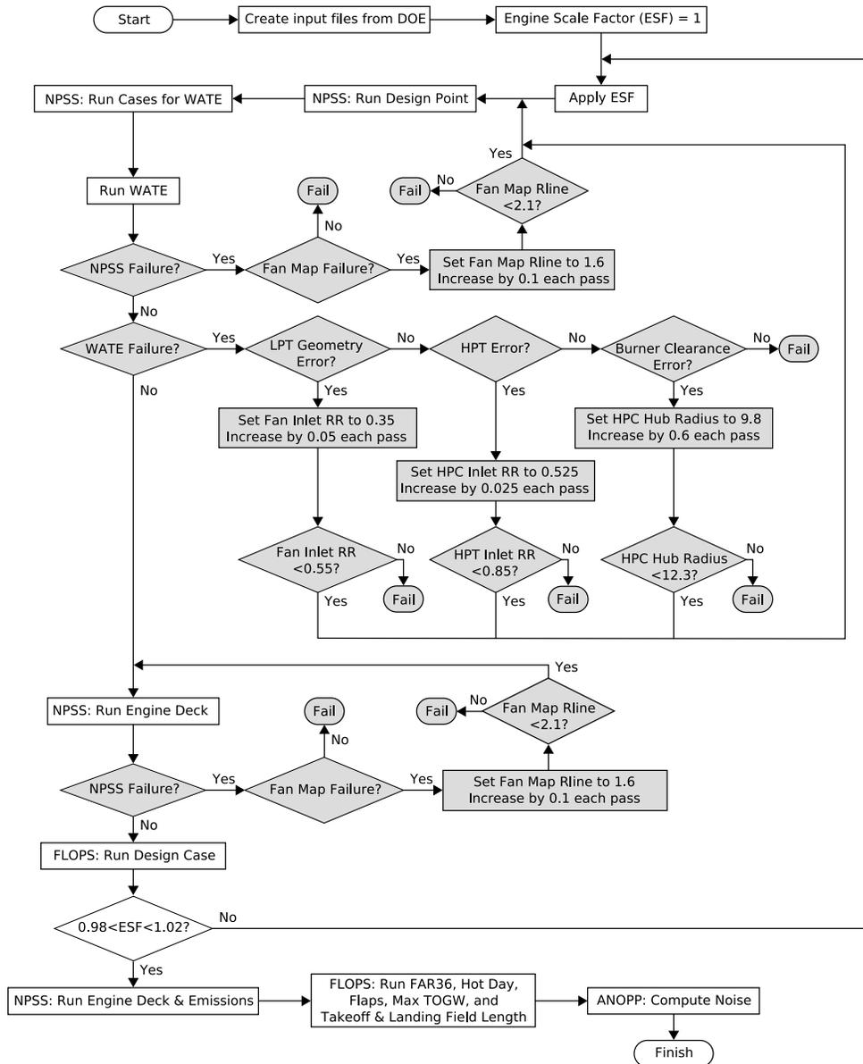
Figure 2-2: EDS Framework Flow Path - White boxes are the main program flow and shaded boxes are error correction steps.
