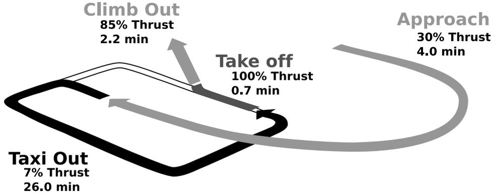
Figure 2-4: Thrust Settings and Segment Times to Measure Airport Emissions[9]
