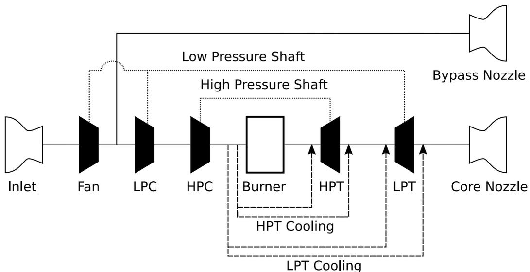
Figure 2-3: NPSS Engine Flow Path Example
