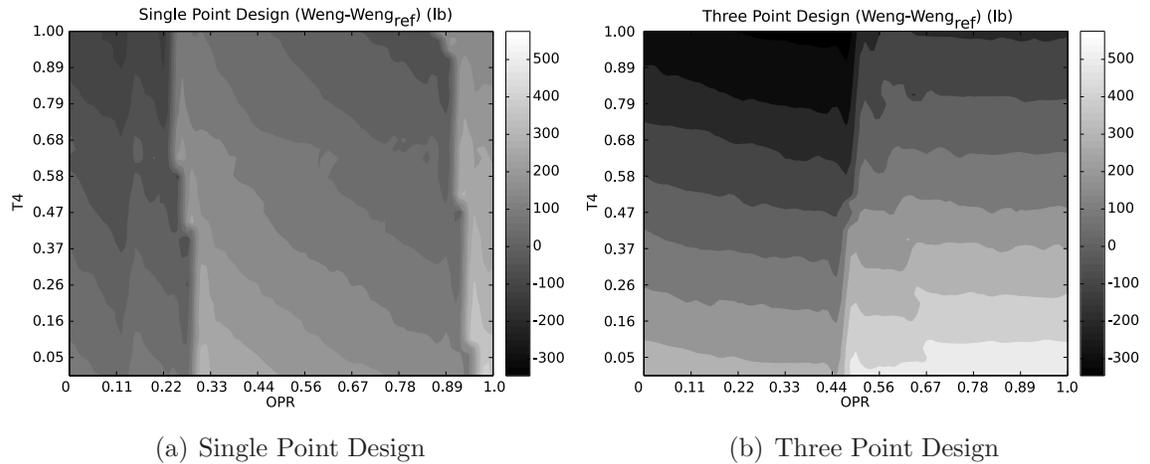
Figure 3-5: Single vs Three Point Design: Bare Engine Weight
