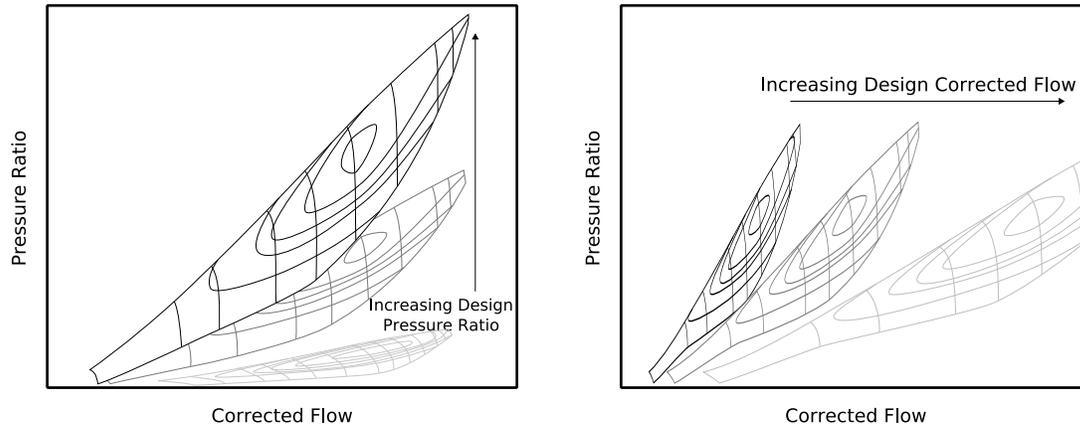
(a) Compressor Map Variation with Design Pressure Ratio (b) Compressor Map Variation with Design Point Corrected Flow
