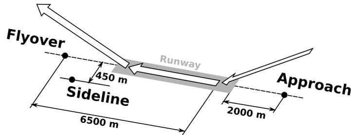
Figure 4-1: FAR 36 Microphone Locations for Aircraft Noise Measurement
